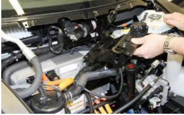
Removing the bracket for the windscreen wiper
