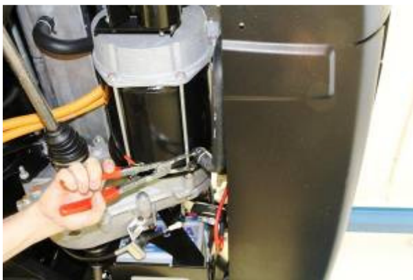
Loosen the clamp for the cooling pipe on engine
